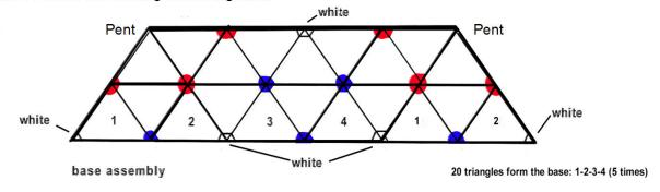
Have you made your models yet? Good! Note: color code goes on inside (not on plywood side) as we erect it from the inside (so as to see it). Paint sides of triangles a little so you can readily identify them when stacked so-- ie. A little color code on the inside and a little on the sides.
