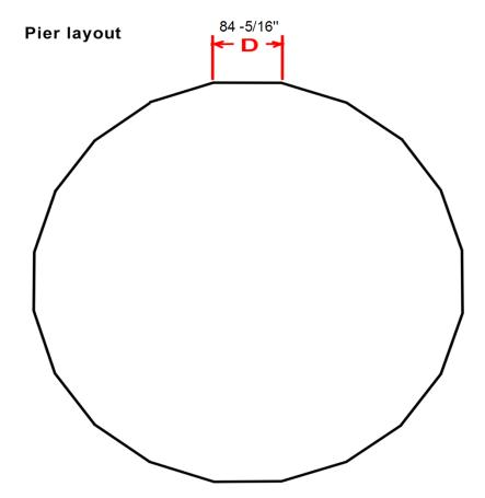
Note: this is an even 20 sided polygon using all "D" strut measurements. (20 vertices x  $18^{\circ} = 360^{\circ}$  or 20 vertices x  $2ea 9^{\circ}$  struts =  $360^{\circ}$ ) If you will be using the polystyrene between triangles and riser wall sections, and because we want the finished outside edge of the concrete to be flush with outside of plywood, add 3/8" to the "D" length.
